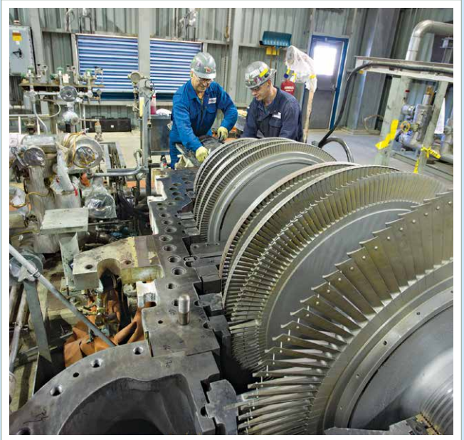
Technicians check tolerances on the steam turbine major equipment to optimize performance for operating reliability and energy efficiency.
